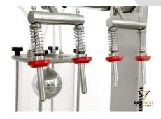
During the work process, operator inserts the bottle into the filling head which then automatically starts filling liquid into the bottle. When the desired liquid level is reached, machine stops the filling process. Liquid level in the bottle is adjusted by setting the filling nozzle. Vacuum bottle filler has 4 filling heads.
