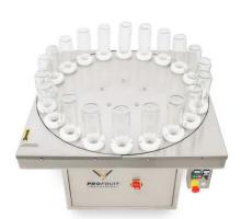
Bottle rinser is a great solution for easily maintaining hygiene standards. The operator manually places the bottles upside down in one of the 20 positions on machine's central plate. The plate is turning in step-by-step motion.
