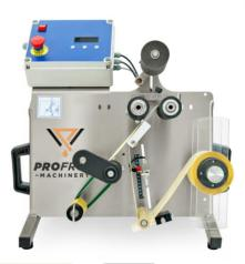
Semi-automatic tabletop single station labelling machine. The front and back self-adhesive labels can be labelled in the same cycle using one bobbin with alternating front and back body label, for cylindrical bottles, glass jars, and other containers. Complete with a LED digital electronic control panel to perfectly centre the labels.
