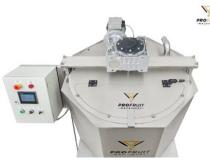
The heating of the product can be done in two ways. The jam cooker can be produced with it's own electric heating elements using glycerin heating instead of water.
