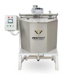
Multi-purpose jam cooker is double-walled and entirely made from stainless steel. Machine has an integrated mixer with specially made scrappers which prevent product from sticking. The jam cooker has adjustable speed as well as fully automatic temperature and cooking time control. The machine also has an integrated touchscreen panel with ability to set the recipes, time, temperature and mixing speed. Therefore, it significantly easies the cooking process and reduces the workload.
