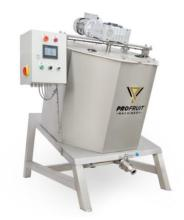
Alternatively, the heating can be done by hot water which can be supplied from our specially made HEAT or ECOHEAT pasteurizers. When heating is done with our jam cooker, you can supply the product into the pasteuriser for a final fast pasteurization in higher temperatures.
