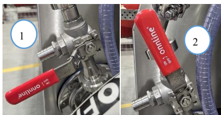
1.10 Fig. Washing ball valve
