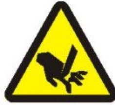
Warning. Sharp parts of machine Risk of limb injury.
