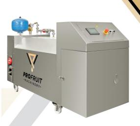
Capacity per hour – 900-1250 L of 80 °C (176 °F) heated juice.
