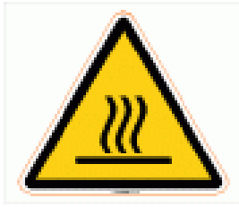
Hot surface. Risk of getting burned.
