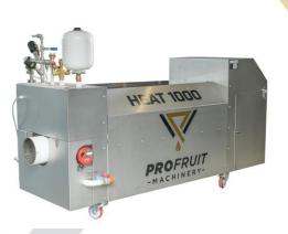
Capacity per hour – 900-1250 L of 80 °C (176 °F) heated juice.
