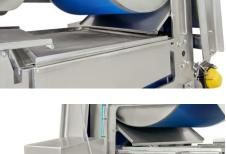
There is a filtration sieve integrated into the juice collection tank. Because of that the belt press 1200 filtrates the juice even during the pressing stage providing cleaner and purer product.
