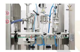
The bottle filling capping machine is perfect to fill various liquids: from water-like to dense food products: juice, milk, puree, jam, marmalade, etc. Machine is ideal for dense and partially dense products – it gives a higher precision in the dosing without pressure adjustments, thanks to the quick electronic adjustment.
