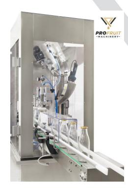
This solution is ideal for small to medium producers of food products, as it allows to work with a speed of about 500-800 bottles/hour, with a minimum manual handling by the operator.
