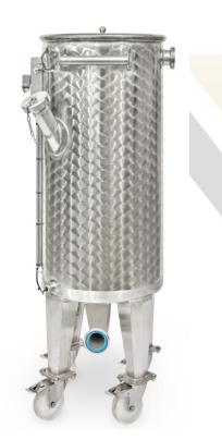
100 L stainless steel tank is used as a buffer tank before the filling process. The tank can be used for storing or mixing the product.
